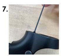
While applying pressure on the spring, install the 6-32 set screw.
