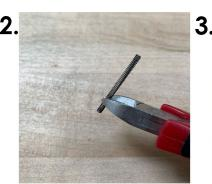
Using diagonal cutters, cut off about 3/16" of one spring.
